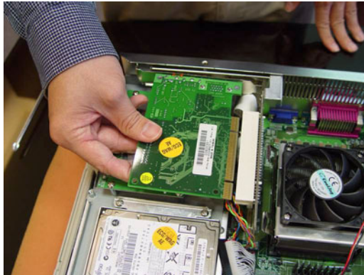
Figure 3.5: PCI bus expansion
